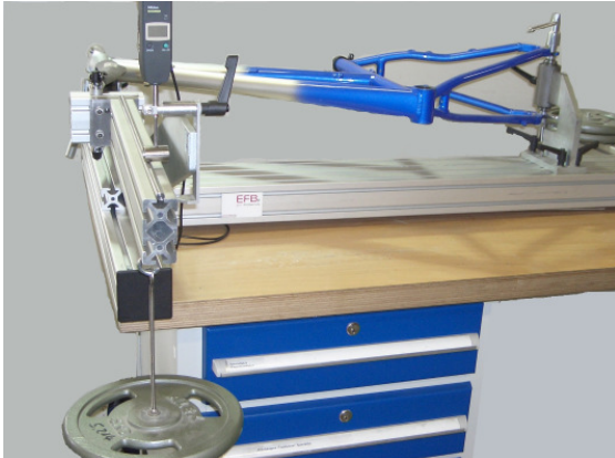
Illustration: Track rigidity testing of complete frame sets
