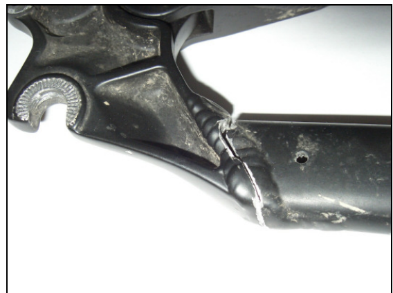
Illustration: Service failure in rear end
