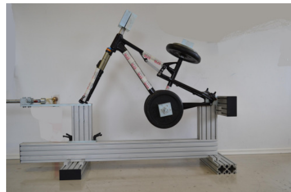
Image: Dropping frame test
